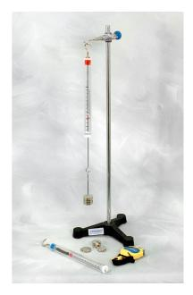
Example of arrangement for Hooke's Law and harmonic oscillations.
